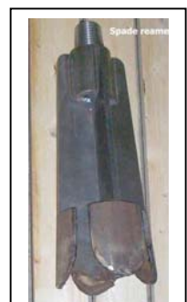
A spade reamer enlarges the hole made by other tools.
